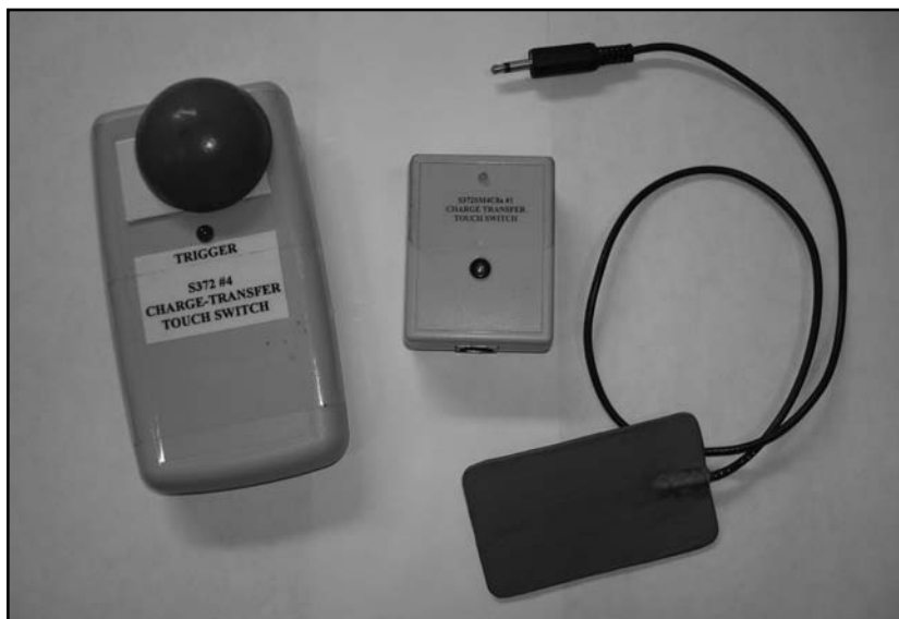
Figure 5-18. Charge transfer/proximity switch.
